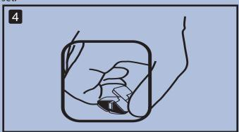
With non-dominant hand, stabilize the port. Do not grasp the vertical fin during removal. This could result in inactivation of the safety feature.
