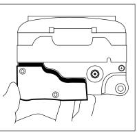
Figure 35. Battery Door Replacement.
