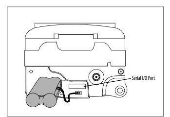
Figure 23. Installation of Battery Pack.
