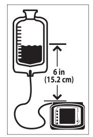
Figure 4B. Correct Fluid Level.
