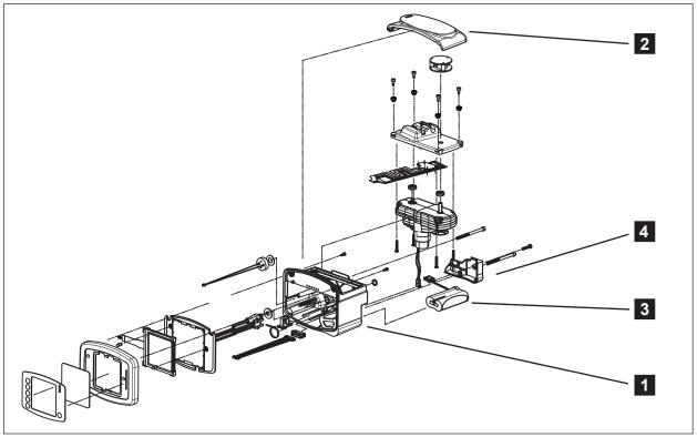
Figure 36. User Serviceable Parts.
