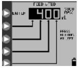
Figure 11C. Setting the Feed Volume to be Delivered.
