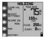
Figure 18A. *HOLDING* mode options, continuous feeding mode.
