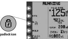
Figure 17. Padlock indicates pump is in *LOCK SCREEN* mode.
