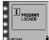
Figure 16. Program Locked screen, which indicates the pump is in LOCK SETTINGS mode.
