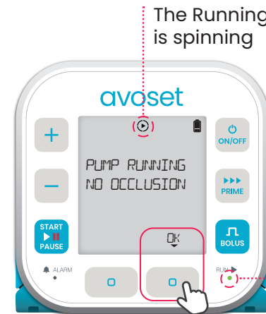
3. The infusion resumes automatically once the occlusion is resolved. Press OK to acknowledge. If the pump doesn't resume
