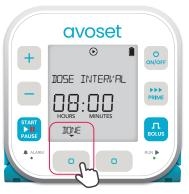
8th parameter: The time between doses. Press the IDNE multifunction button to navigate to the main display
