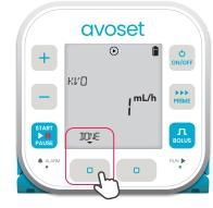
8th parameter: The Keep Vein Open rate. Press the IONE multifunction button to navigate to the main display
