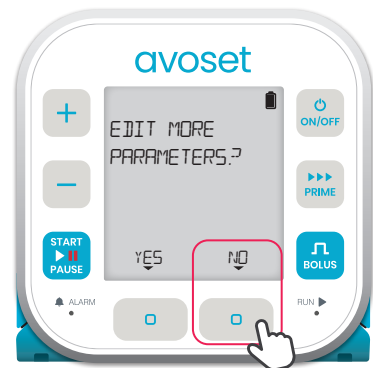
5. To edit additional parameters press the YES multi-function button, to finish editing press NO
