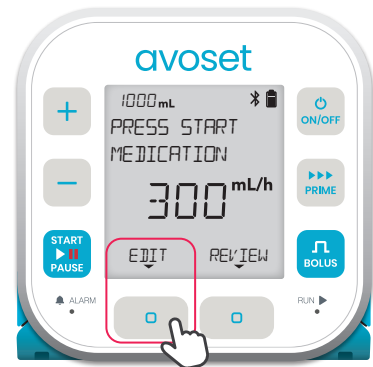
1. Press the EDIT multi-function button to change infusion parameters
