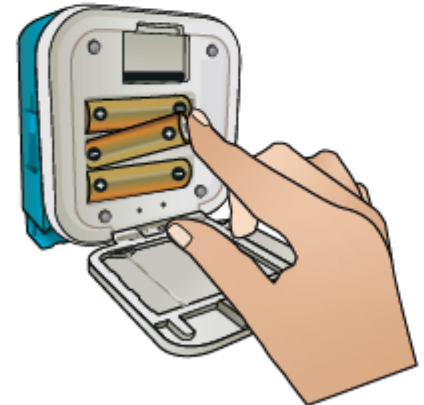
4. Remove each battery starting with the positive (+) ends
