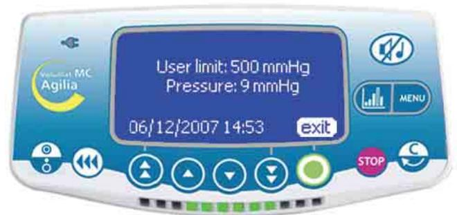
This screen appears when pressing the eye key. User limit indicates the limit set by the user. Current limit is the pressure on infusion in the line.
