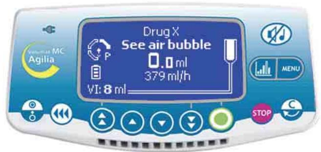
**Note:** This feature is available only when an **air alarm** is triggered (air volume exceeded or air bubble in front of the air detector). The air bubble is removed without having to open the pump door.
