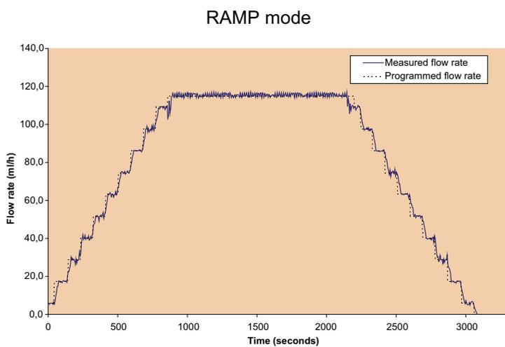
Ramp up: 15', ramp down: 15', stabilized flow rate: 115 ml/h, total volume: 70 ml.
