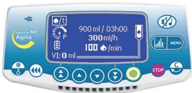
This infusion mode allows to convert the traditional prescription of rate in drops per minute into flow rate in ml/h.
