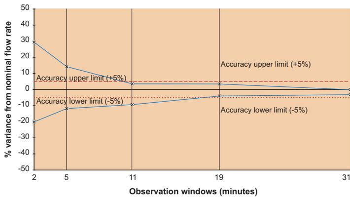
Flow rate/Time curves: start-up and instantaneous flow rate (volume is measured every 30 seconds)
