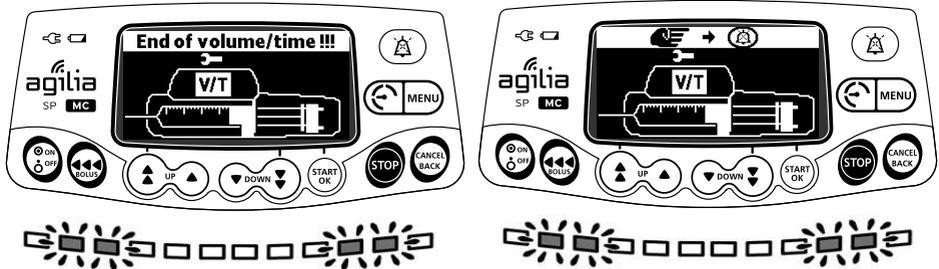
**Figure 7.3:** End of Infusion with KVO Disabled, Continuous Disabled (End of Volume/Time)
