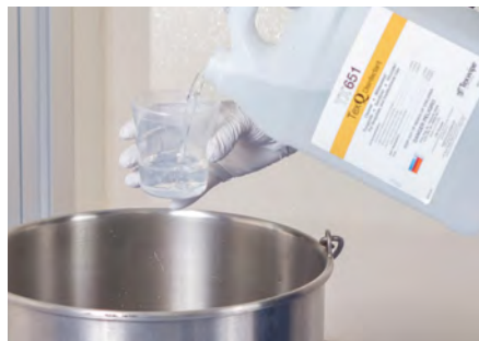
Measure the TexQ® disinfectant TX651 using the supplied (included) beaker, 2 oz. per gallon of water.
