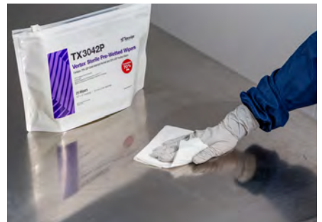
Remove any remaining residue with an isopropyl alcohol (IPA) pre-wetted wiper.
