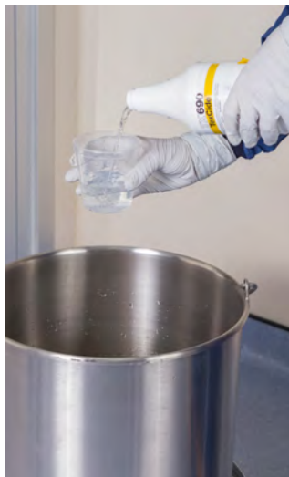
Measure TexCide™ disinfectant TX690 using the supplied (included) beaker, 4 oz. per each gallon of water.
