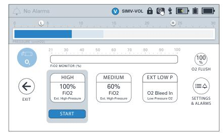
monitor to ensure the accuracy of delivered Oxygen therapy whenever the FiO2 control is used.
