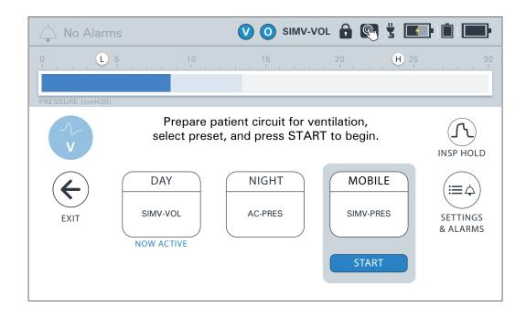
NOTE: To change Ventilation therapy settings press the Preset name and then the SETTINGS & ALARMS button. Follow the instructions described in *"Changing Ventilation Therapy Settings" on page 64* to modify Ventilation therapy settings. When configuration is complete, press < EXIT to return to the Ventilation therapy screen.
