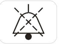
NOTE: The Internal Battery Critically Low alarm cannot be silenced until VOCSN is plugged into an external source of power. To silence the alarm after plugging in VOCSN, access the Alarm Log (by pressing the alarm banner in the upper left-hand corner of the screen or pressing LOGS in the Menu tab), and then select CLEAR LIST.
