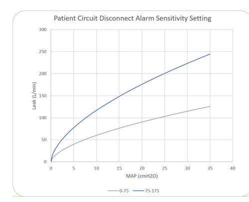
The graphic to the left shows how the SENSITIVITY setting interacts with leaks at various Mean Airway Pressures (MAPs):
