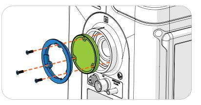
CAUTION: Do not let anything enter the cavity behind the filter during the replacement process. Do not re-install the Internal Bacterial Filter screws without using a calibrated torque driver. Foreign material inside VOCSN or using too much torque on these screws may severely damage VOCSN.
