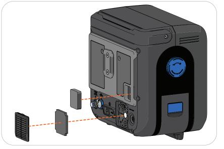
Inspect the filters for signs of damage or contamination. Replace the filters if they appear damaged. Repeat the cleaning steps described above until the filters pass a visual inspection for cleanliness.
