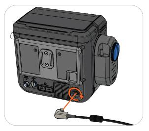
The 24 Volt Wheelchair Power Cable comes with a hook-and-loop strap to manage excess cabling. Coil extra cabling between the outlet and VOCSN, and then wrap the strap around the cabling to secure it.
