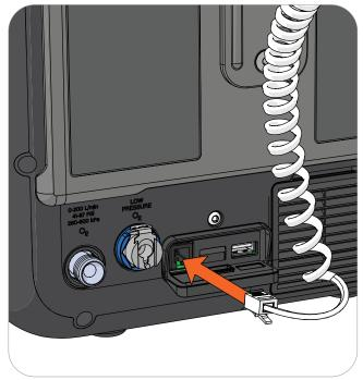
WARNING: To reduce the risk of electrical shock, ensure the Nurse Call System connected to VOCSN meets the Safety Extra Low Voltage (SELV) requirements as described in IEC 60601-1 (1988).
