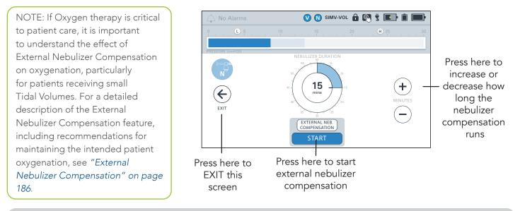
WARNING: Use only 6 L/min nebulizer cups with VOCSN. VOCSN ventilation compensates for 5.9 L/min of nebulizer flow. When gas is added to the Ventec One-Circuit from a nebulizer producing a flow less or more than 6 L/min, the accuracy of delivered ventilation may be temporarily affected.
